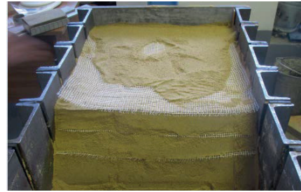
b. Reinforced elements (geogrid)
